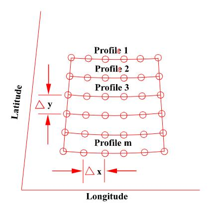
Figure 1 Structure of digital elevation data, arc-second grid.
