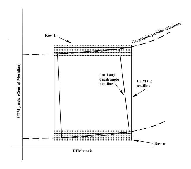
Figure 2 Structure of digital elevation data, UTM meter grid
