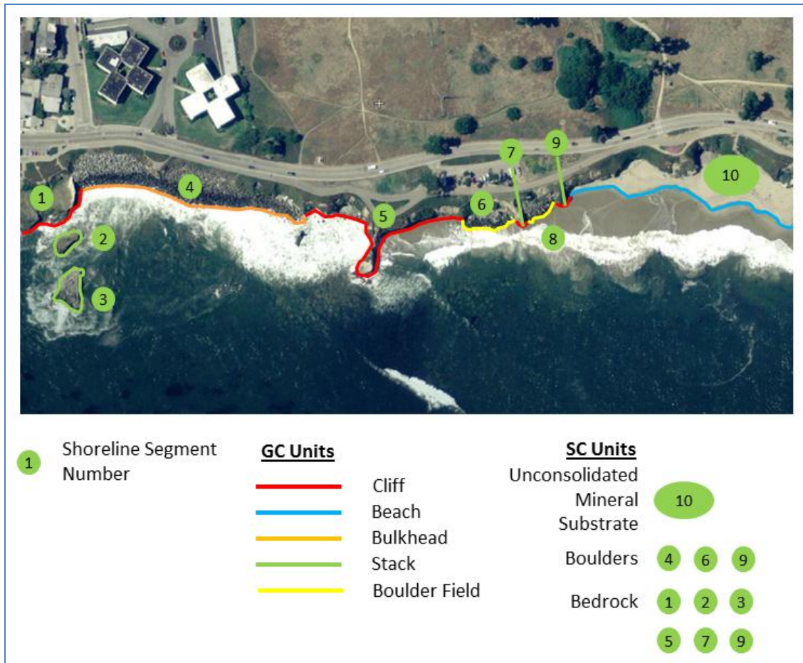
Figure 12.2. Shoreline Characterization. California coast, showing GC units as segments with Substrate Component attributes.
