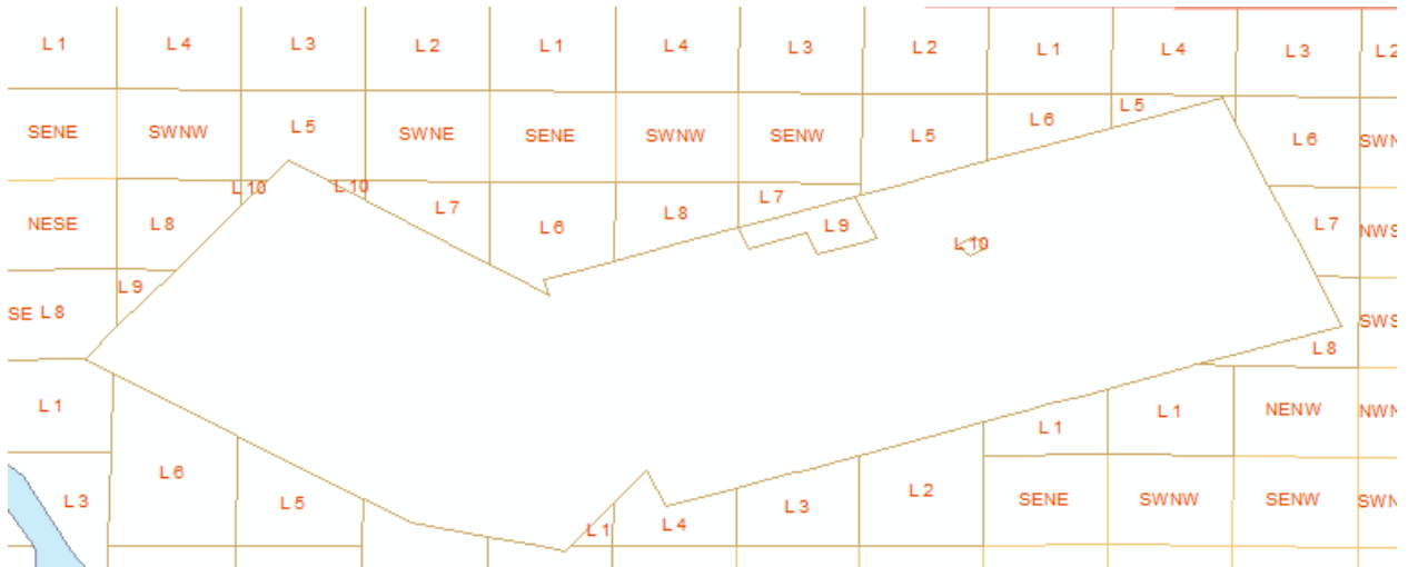
Figure 10 - Apparent "Hole" is Rectangular PLSS
