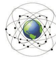
BeiDou 6 Orbital planes 35 Satellite + 3 GEO + 27 MEO + 3 IGSO 55° Inclination Angle Altitude 38,300 km, 21,500 km
