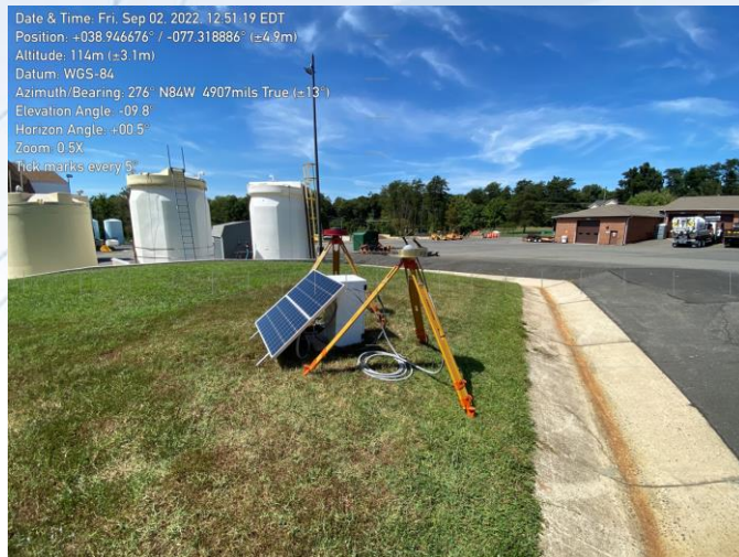
T-CORS at Virginia DoT Reston Road Yard (<200 m from Ligado HQ)
