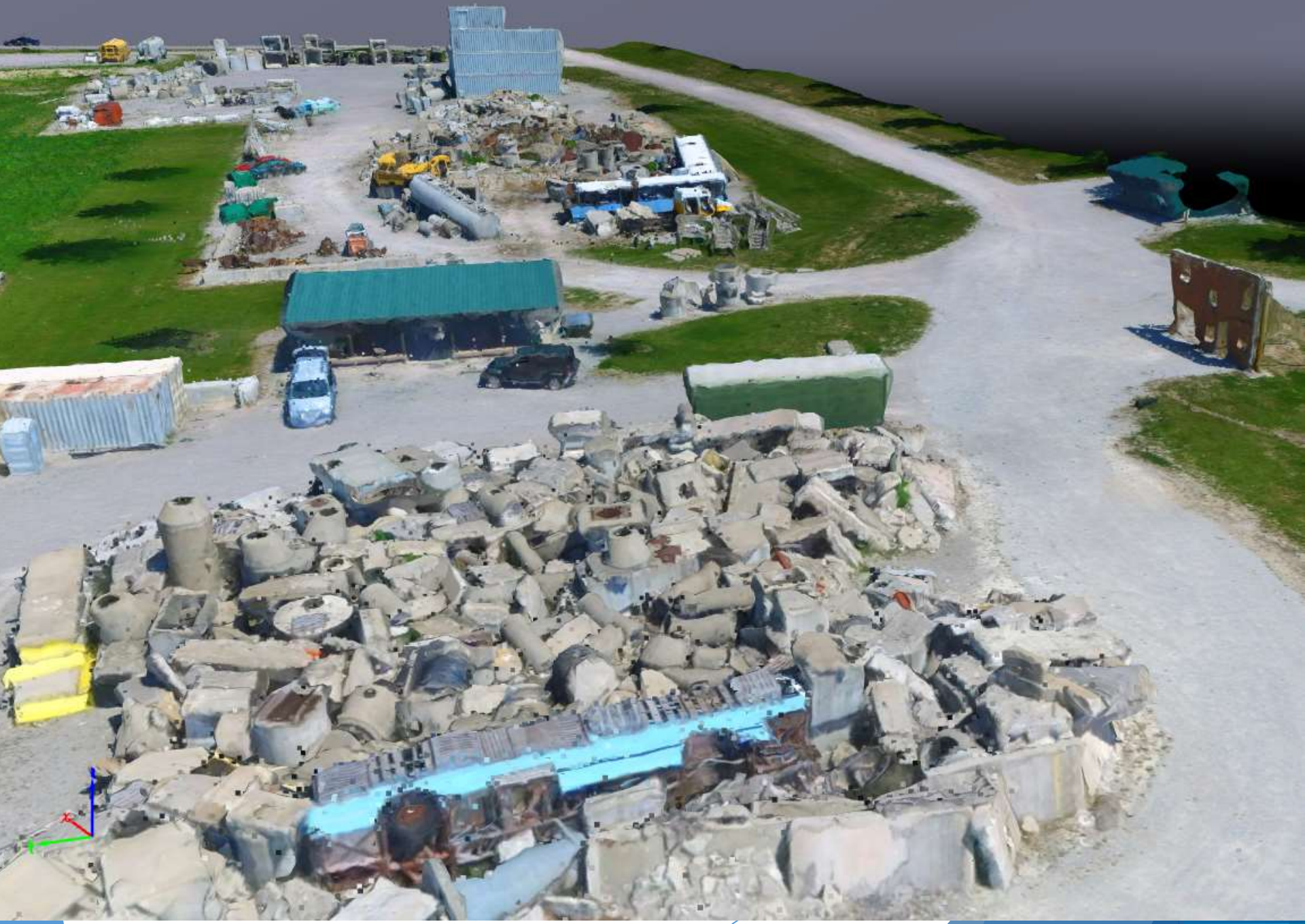
3D Triangle Mesh from ~34,000,000 Colorized Point LAS Cloud
