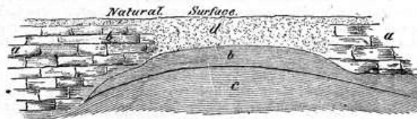
FIG. 25. CRETACEOUS CLAY BENEATH THE SHAKOPEE LIMESTONE, MANKATO. a. Shakopee limestone. b. Bedded greenish clay, weathering white, but little sandy. c. Sandy, bedded greenish clay. d. Drift, mostly coarse fragments of Shakopee limestone.
