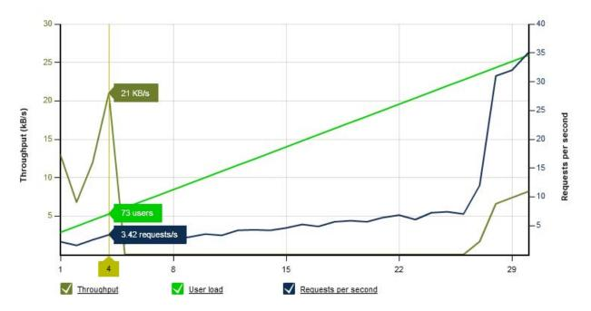
Figure 7 - Initial Amazon Heavy load test (terminated early due to unresponsiveness)
