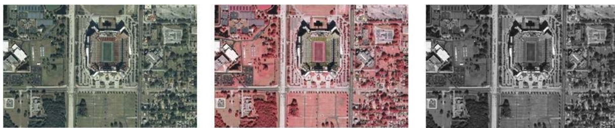
Figure 4: (From left to right) Natural Color, False Color Infrared, and Black and White
