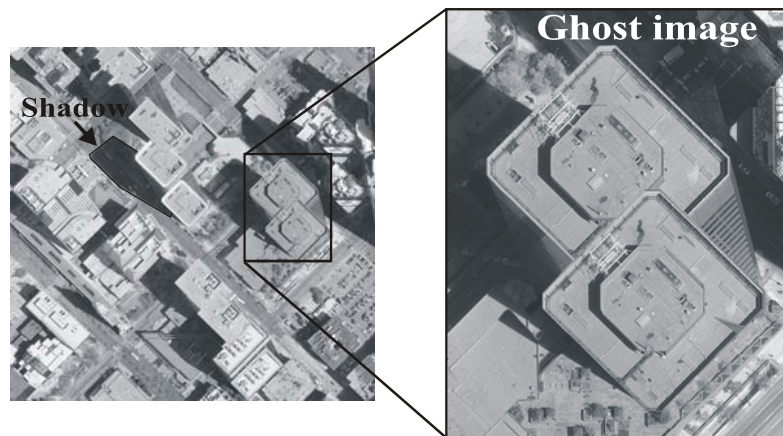
Figure 2 Part of the orthorectified image of downtown Denver generated by the differential model
